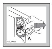
Remove the security gasket cup by turning and pulling it away. Pay attention not to move or remove the gasket.
